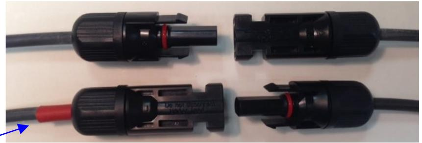
Each CyboInverter has 4 pairs of MC-4 DC connectors. The red labeled wire is “+”. Plug in each pair of the MC-4 connectors to its corresponding solar panel.
