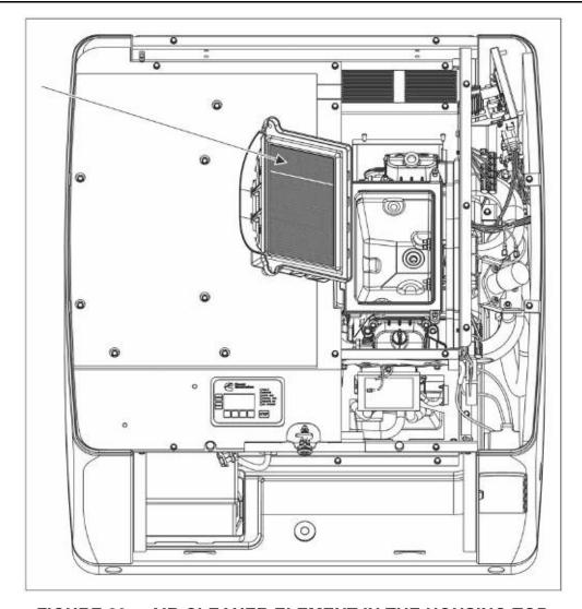
FIGURE 38. AIR CLEANER ELEMENT IN THE HOUSING TOP
