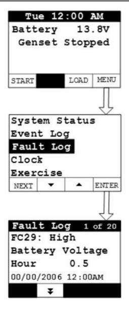
FIGURE 13. FAULT LOG SCREEN
