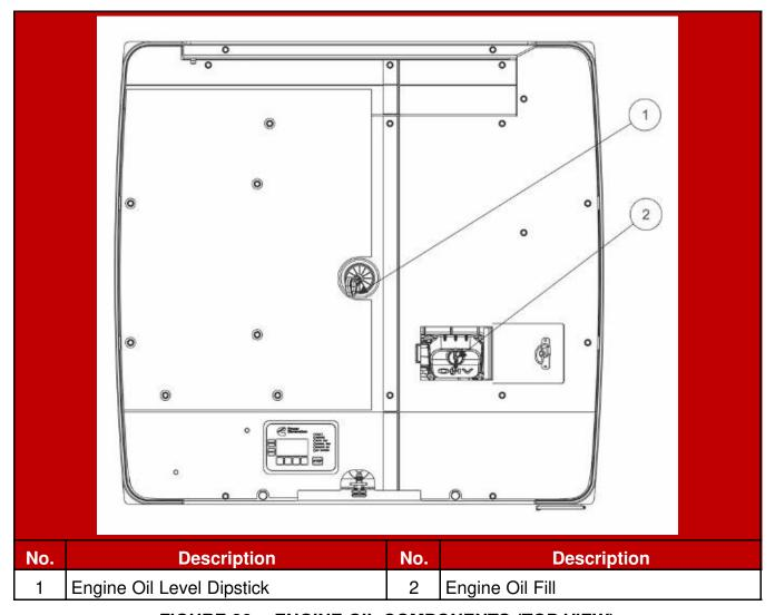
FIGURE 36. ENGINE OIL COMPONENTS (TOP VIEW)
