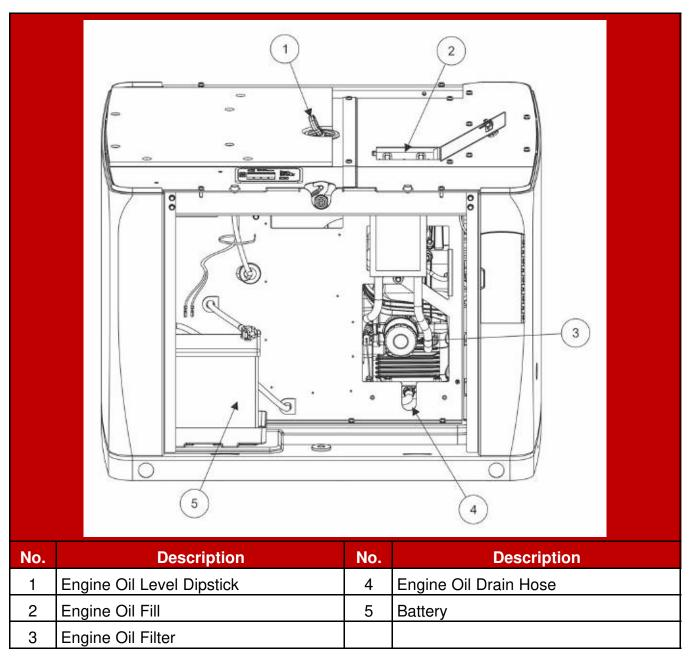
FIGURE 35. ENGINE OIL COMPONENTS (SIDE VIEW)
