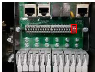
Fig. E – Dipswitch Location on 15K
