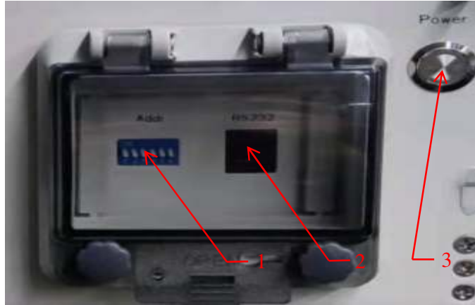
Figure 2.4. Battery module interface definition
