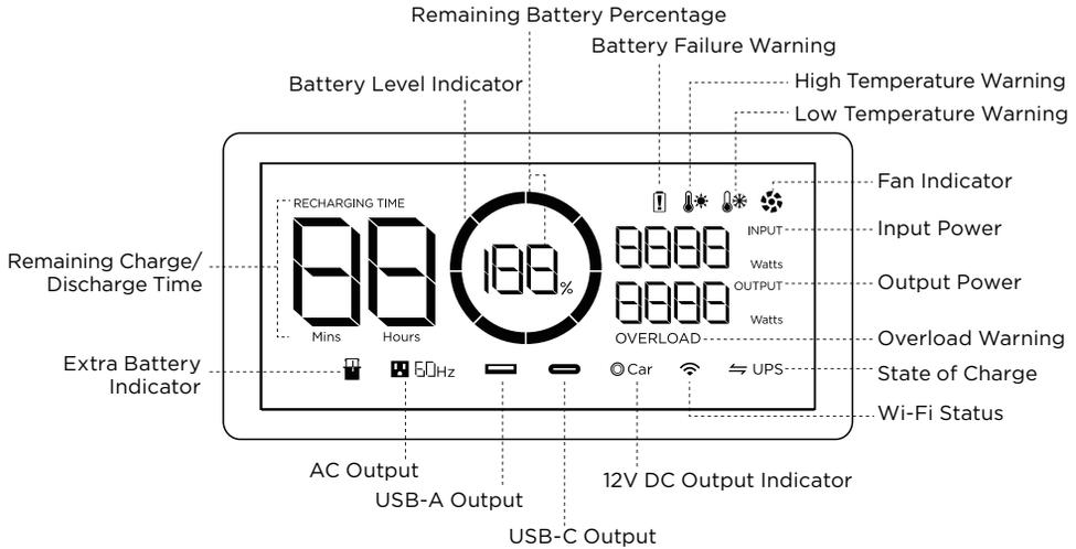
**Battery Level Indicator:** The indicator will repeatedly fill while charging. If product is at 0% charge, the indicator will flash to warn you.
