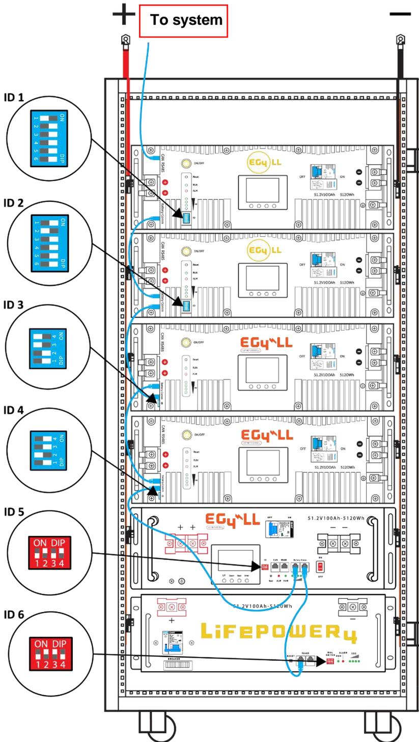
1. Always use the newest model of LL at the top of your rack as this will need to be the battery that communicates with the system. This battery is also known as the master and will need to have ID number 1.
