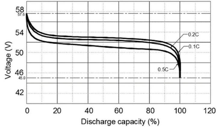
Charge & Discharge curve with 0.5C @ 25°C
