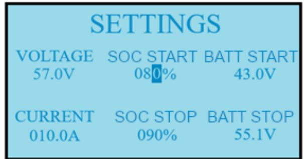
Press the "DOWN" button to highlight the BATT START setting and repeat the steps above to make and save changes to the BATT START parameter.
