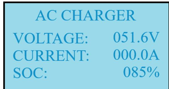
The main screen will display “LOST” for the SOC value when the charger is not connected to a battery via RS485 and is not receiving SOC data.
