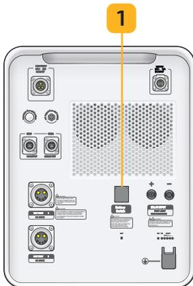
1. With all cables disconnected, press the **Battery Switch** to connect the battery. Touchscreen will light up.
