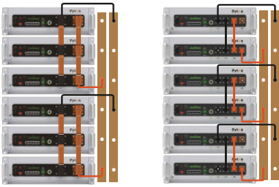
Figure 5-1 Schematic diagram of power cable connection
