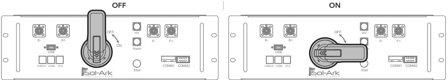
Figure 14 Operation of the BMU DC Disconnect
