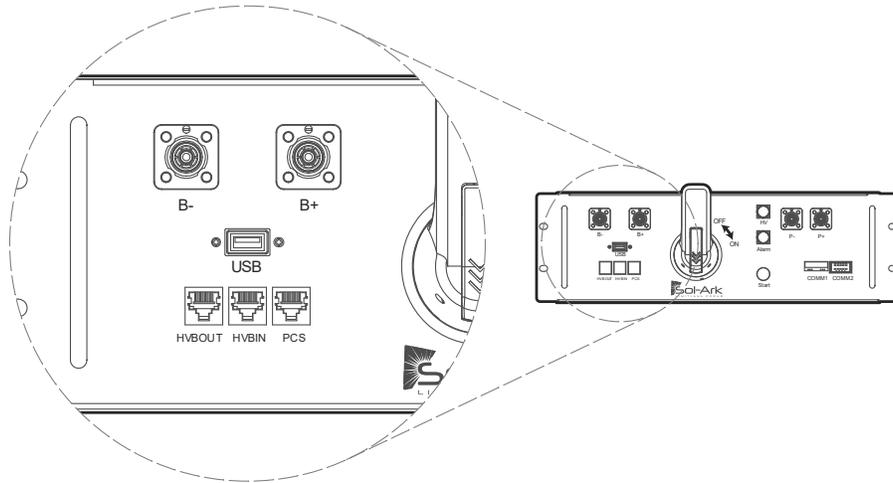
Figure 15 Close up of USB upgrade port
