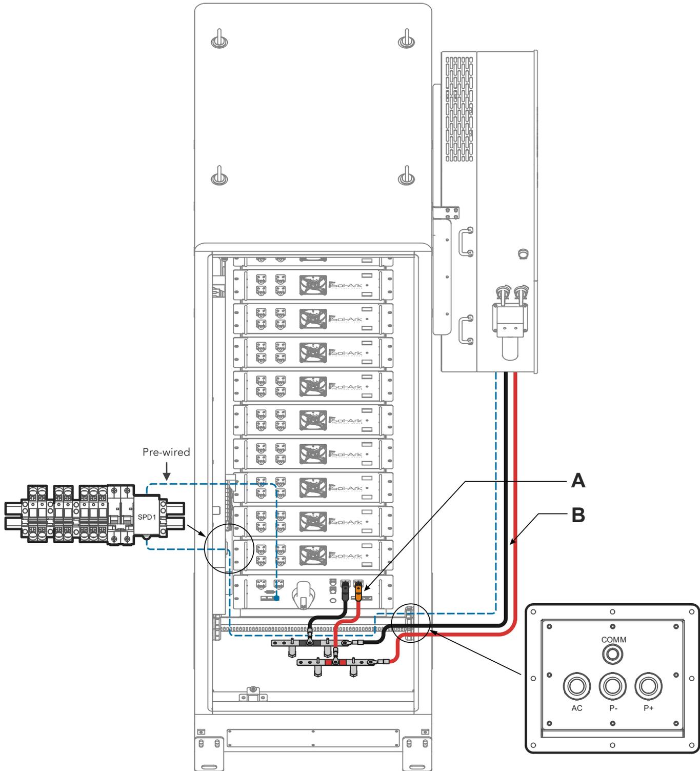
Figure 10 Wiring of the cabinet to the inverter
