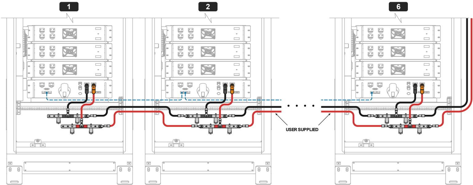
Figure 11 Illustration of wiring for a multi-cabinet system.
